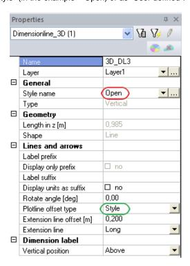
You change Plotline offset type to "User defined" and you can see the changes in the image of the dimension line. There is a new row in the properties. You can define a new plotline offset by number in this new row.
