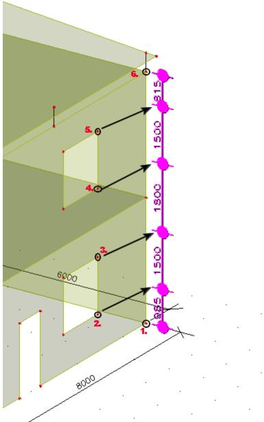
7) Continuous dimension line behaves like one item with its own properties. You can divide a continuous dimension line to single dimensions. The tool for this operation is "Break dimLine to single dimLine"
