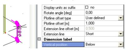
The extension line is non-editable. Extension line type "Short" has a default offset which is changed according to the Plotline offset. It always displays a short extension line. See example with Plotline offset 2m (picture below). You can see the difference from the extension lines offset which is defined by the Plotline offset value 1m (picture above).
