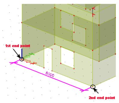
4) You insert dimensions also in the Y and Z direction in the same way as in the X direction. You just need to use proper Dimension tools – the one with little Y and little Z and little Z and little Z., respectively.
